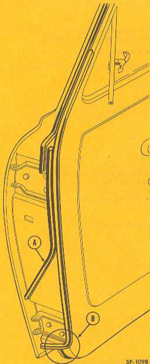
Fig. 3 - Weatherstrip Installation at Front of Door
