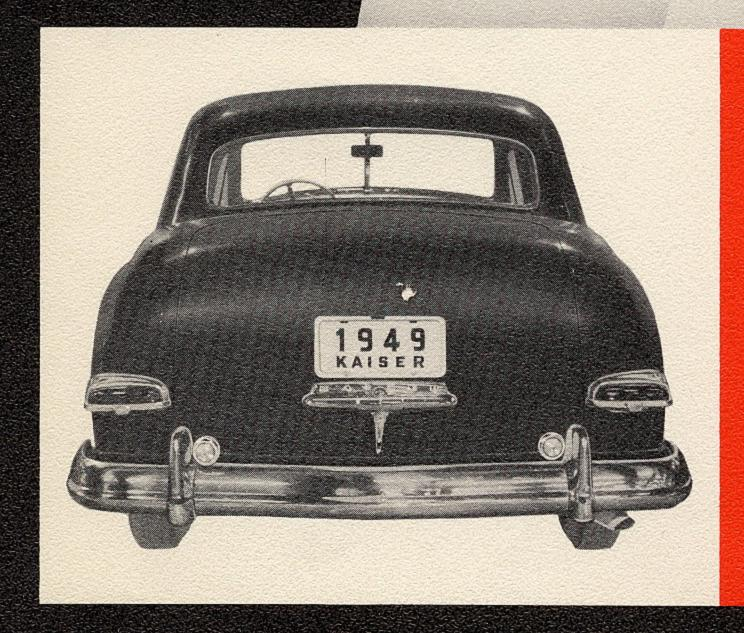
Back-Up Lights are installed on the rear bumper guards. Because of the guard locations, the same lamp is used as left hand on the Kaiser and right hand on the Frazer, while the right hand Kaiser is the same as the left hand Frazer.
