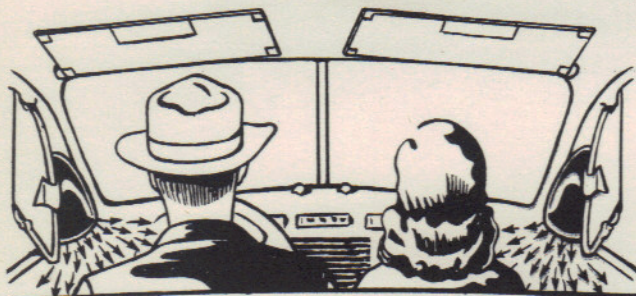
Circulates cool outside air forcing out super-heated air.
