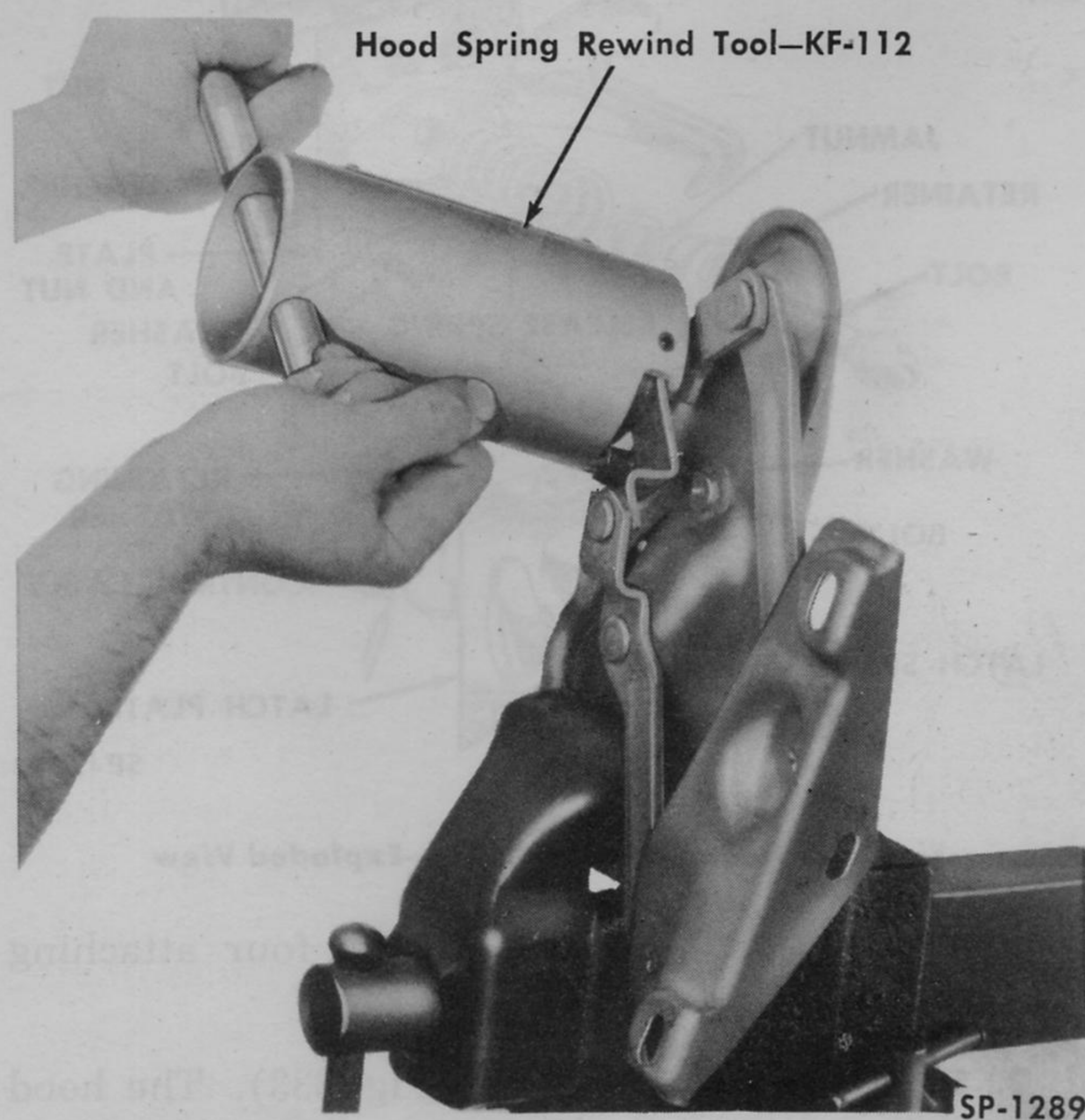
Fig. 336—Replacing Hood Hinge Spring—Kaiser
